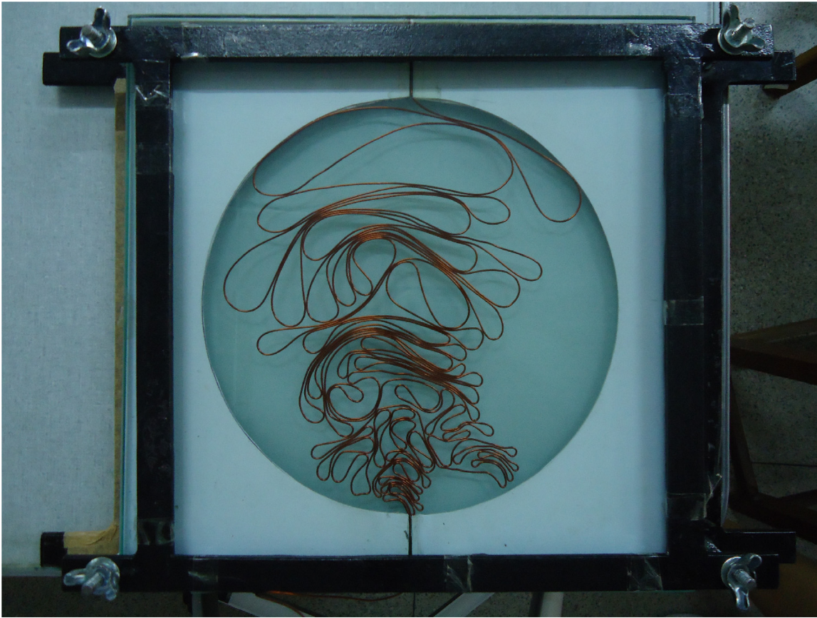
Fig 1. A wire that is 5020 mm long at the jammed state in a circular cavity whose diameter is 22 cm. Our experiment consists in measuring the force needed to pull that piece of copper outside the cavity.
